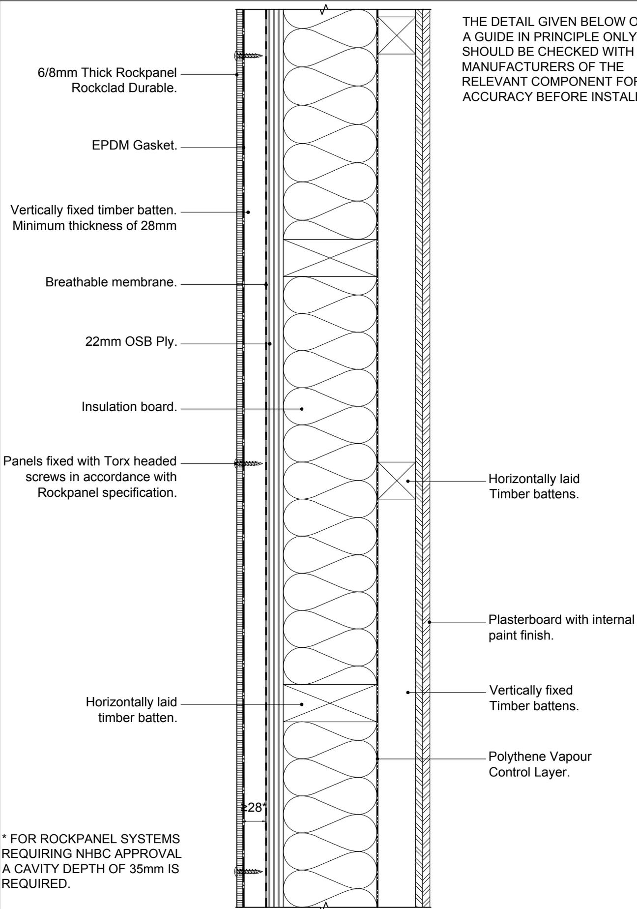
\* FOR ROCKPANEL SYSTEMS REQUIRING NHBC APPROVAL A CAVITY DEPTH OF 35mm IS REQUIRED.
