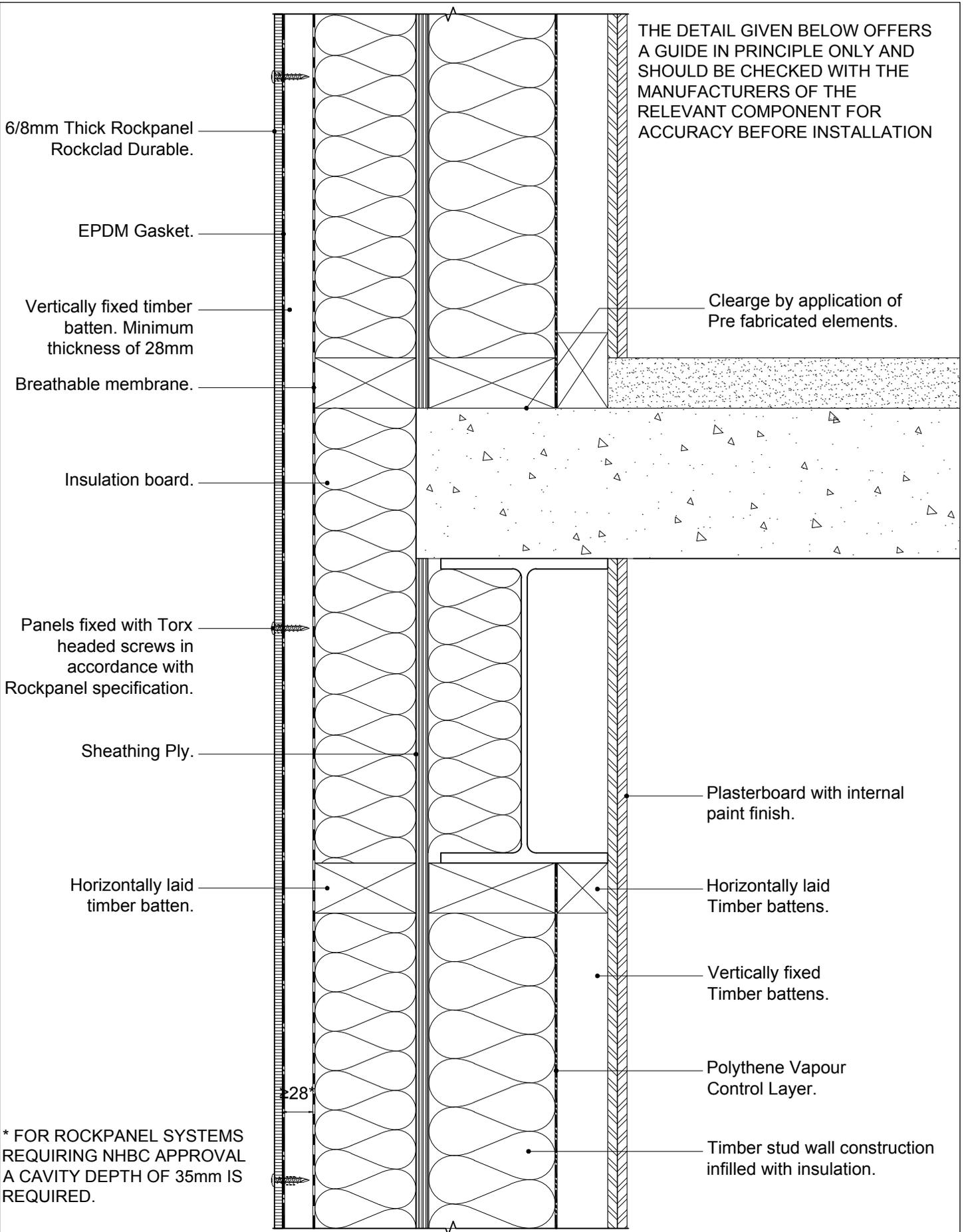
**DETAIL 7 - ROCKCLAD DURABLE VERTICAL SECTION TIMBER SUBSTRUCTURE TO STRUCTURAL STEEL WITH TIMBER STUD FRAME.**
