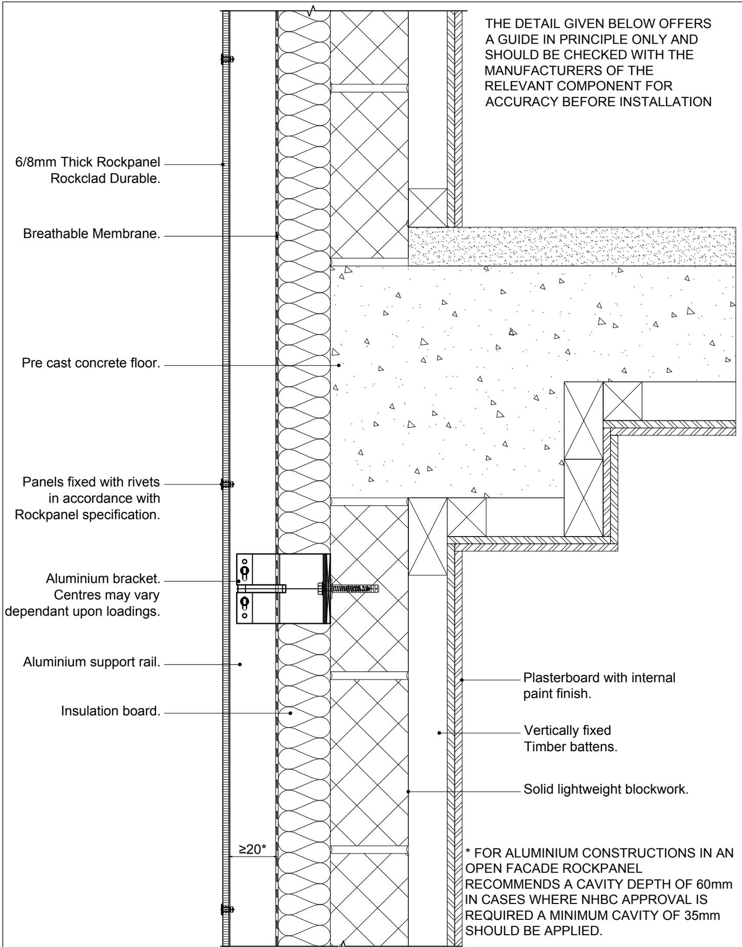
\* FOR ALUMINIUM CONSTRUCTIONS IN AN OPEN FACADE ROCKPANEL RECOMMENDS A CAVITY DEPTH OF 60mm IN CASES WHERE NHBC APPROVAL IS REQUIRED A MINIMUM CAVITY OF 35mm SHOULD BE APPLIED.
