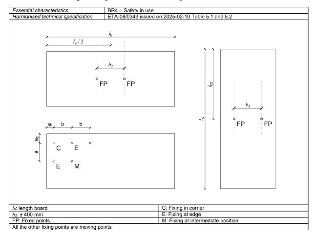
Table 7 - Performance shear strength mechanical fixings
