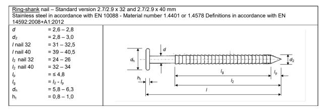
Table 8b – Specifications mechanical fixings – fasteners for timber sub-constructions.
